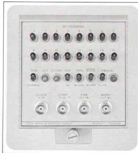
Fig. 1. Characters are generated by setting the appropriate toggle switches on the front panel of this HP Model 1925A Word Generator plug-in. Complement, pseudo-random noise, and RZ and NRZ formats can be selected.
