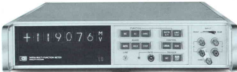
Fig. 4. Basically a five-digit integrating DVM, the HP Model 3450A measures dc voltage and voltage ratios. With plug-in options, measurement capabilities including ac, ohms, limit tests, digital output and remote control may be added.
