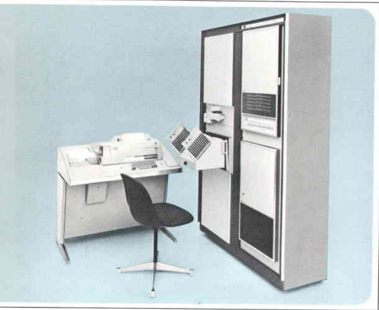
Fig. 1. Model 2060A Digital Logic Module Test System can give most production logic modules a thorough functional test in less than 30 seconds. It is programmed in AuTest, a special simplified language. Once programmed, it can be used by unskilled operators.
