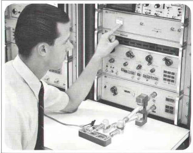
Fig. 2. The thin-film amplifier in the foreground is about to have its s -parameters measured automatically by the HP 8541A Automatic Network Analyzer, a computer-controlled system programmed in BASIC or FORTRAN. Programs for performing many tests are supplied with the system. Special tests are programmed by the user.
