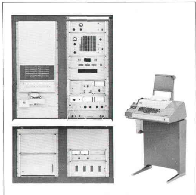
Fig. 4. The HP 9500A is a computer-controlled system designed to test a variety of electronic components, modules, and assemblies, over a frequency range of dc-500 MHz. It provides stimuli, measures responses, processes data, and records results, all automatically. It is programmed in HP BASIC.
