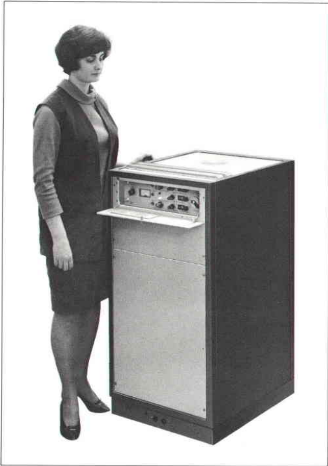
Fig. 5. The latest version of the hydrogen maser is much smaller and more rugged than previous designs. Two masers similar to this one but without cabinets will be put into orbit in a satellite to test the gravitational red shift predicted by Einstein.
