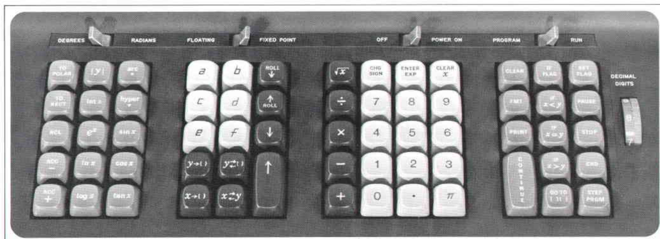
Fig. 4. Keys are in four groups on the keyboard, according to their function.
