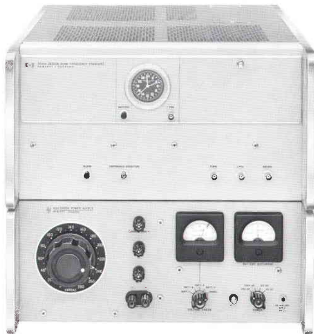
Fig. 1. Atomic-controlled cesium beam frequency standard and clock assembly, complete with standby battery power supply, as used in 1967 Hewlett-Packard flying clock time comparisons.
