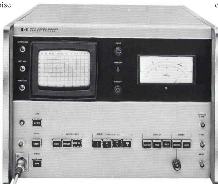
Fig. 1. New HP Model 8051A Loudness Analyzer measures loudness of narrow-band or wideband, continuous or impulsive sounds. Analyzer makes Zwicker-type analysis, gives results which agree well with subjective sensation of loudness. CRT shows loudness density versus subjective pitch; meter shows total loudness.
