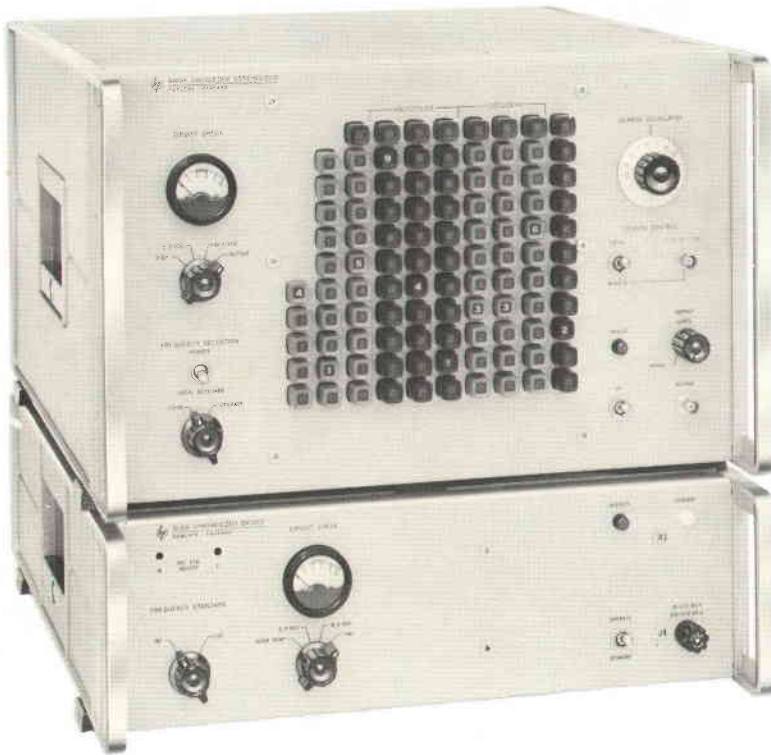
Fig. 1. Pushbutton bank on the HP Model 5105A Frequency Synthesizer permits selection of high-quality signals up to 500 MHz in steps as fine as 0.1 Hz increments.
