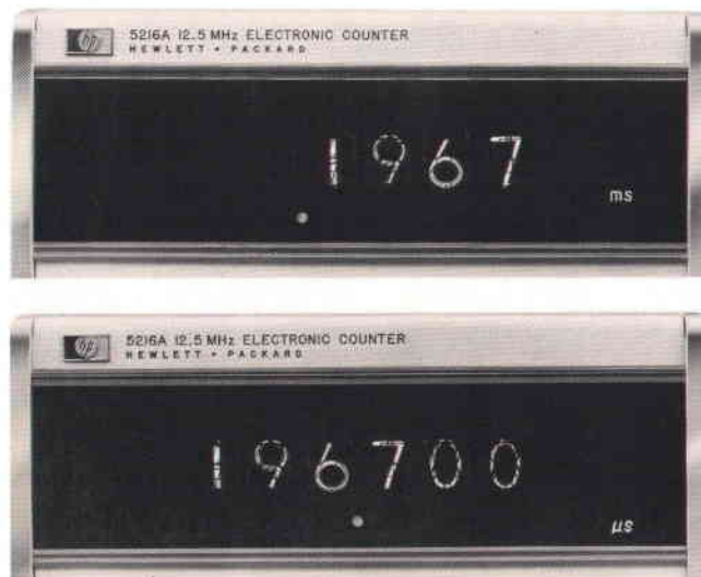
Fig. 3. Zero-suppression feature of new IC counters makes digits at left of display dark when not in use. Older counters showed zeros in these columns and were harder to read.
