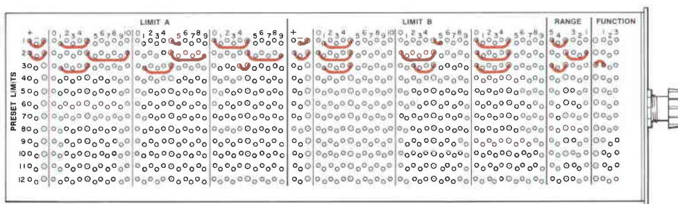
Fig. 5. Up to 12 tests may be preset using the programmer plug-in. Upper and lower limits, polarity, range and function are set up using jumper wires.
