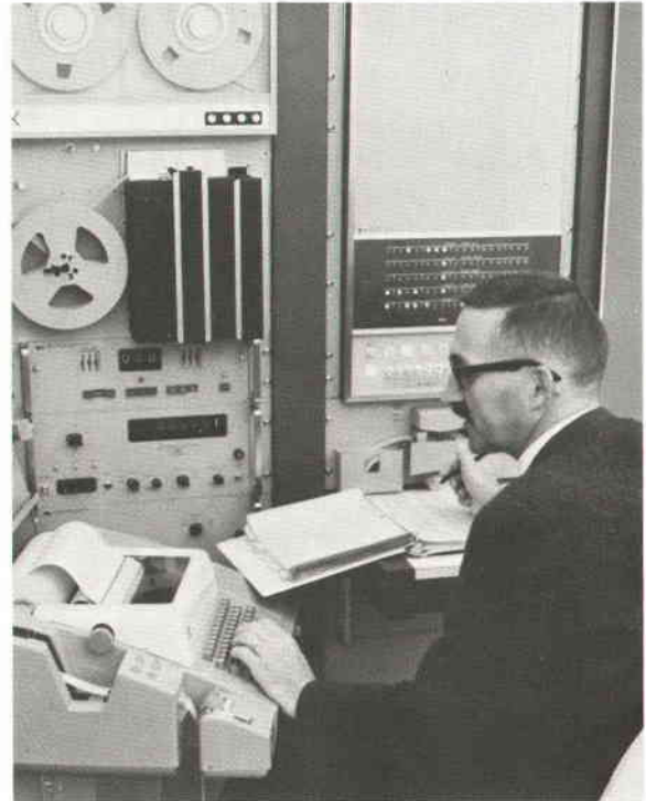
Fig. 1. Computing data acquisition system can be used in a variety of scientific and industrial applications, including jet engine testing (see Fig. 2).
