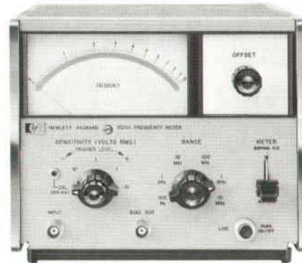
Fig. 1. New -hp- Model 5210A Frequency Meter and FM Discriminator directly measures frequencies between 3 Hz and 10 MHz. Special log-linear meter scale can be read accurately within \pm 1\% of reading. Discriminator output is useful for measurements of instantaneous frequencies of FM signals, measurements that are impossible for most other frequency measuring devices.
