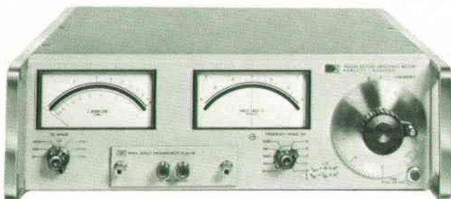
Fig. 1. This low-frequency -hp- Model 4800A Vector Impedance Meter makes rapid measurements of components and circuits with direct read-out over the frequency range from 5 Hz to 500 kHz, and over the impedance range from 10 ohms full scale to 10 megohms full scale.
