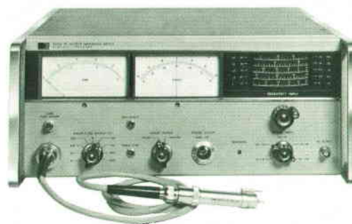
Fig. 5. In-circuit measurements of both active and passive devices and circuits can be made and read out directly over a frequency range of 500 kHz to 108 MHz with the new -hp- Model 4815A RF Vector Impedance Meter.
