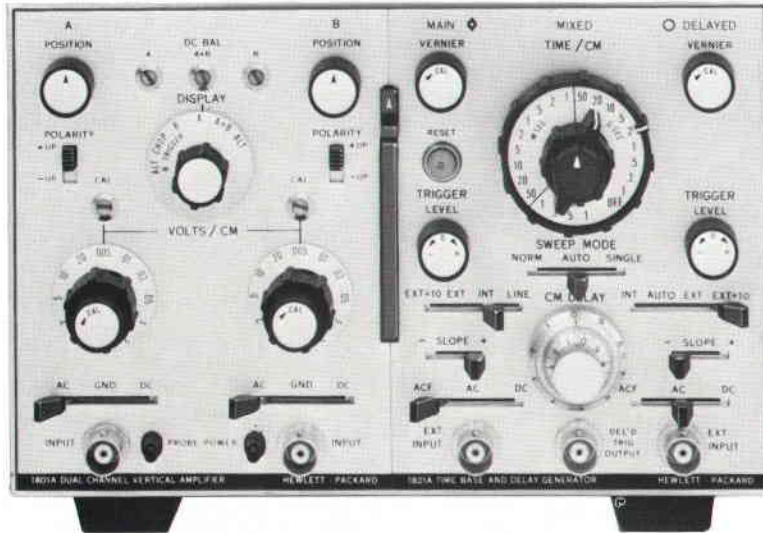
Fig. 9. Controls on the plug-ins are grouped according to function. Vertical amplifiers are in the plug-in at the left and channel controls are arranged vertically with the display control in the center. The horizontal sweep plug-in at the right includes sweep delay.
