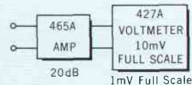
Fig. 10. A 10 mV voltmeter such as the -hp- Model 427A can be extended to read 1 mV full scale with the amplifier gain set at 20 dB.
