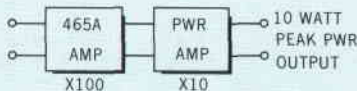
Fig. 9. Cascading the -hp- 467A Power Amplifier with the amplifier results in a stable 60-dB amplifier with 10-megohm input impedance and 10 watts peak power output.
