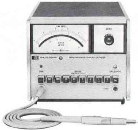
Fig. 2. Broadband sampling voltmeter, -hp- Model 3406A, has 50- \mu V sensitivity, 20- \mu V resolution, flat frequency response from 10 kHz to 1 GHz. Accuracy is \pm 3\% to 100 MHz, \pm 5\% to 700 MHz, \pm 8\% to 1 GHz. Sampling circuit output is available on rear panel, giving instrument unusual capabilities for analysis of broadband signals.
