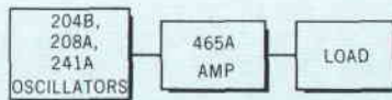
Fig. 8. Output of low power test oscillators can be increased sufficiently to drive a loudspeaker if desired.
