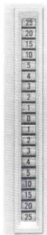
Fig. 9. Position of zero level baseline selected by Positioning control is indicated by illuminated numerals, enabling measurement of dc levels with analog voltmeter accuracy even with zero level displaced up to \pm 25 cm from center screen.
