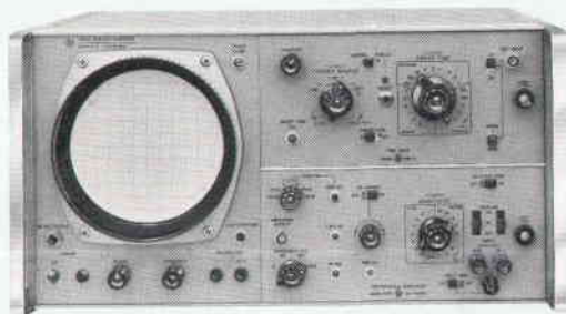
Fig. 1. New -hp- Model 1407A Differential Amplifier Plug-in (in lower plug-in compartment) works with either Model 140A General Purpose Oscilloscope or Model 141A Variable Persistence Oscilloscope. DC stabilization of plug-in amplifier eliminates drift problems, enabling use of dc coupling with deflection factors as low as 50 \mu V/cm. Plug-in has upper frequency limit of 400 kHz.
