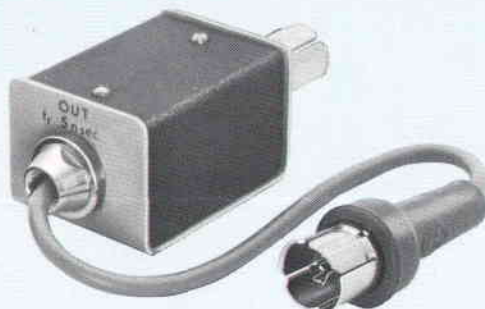
Fig. 1. New rise time converters, -hp- Models 10452A to 10456A, slow the rise time of the voltage step in the -hp- TDR system to 0.5, 1.0, 2.0, 5.0, or 10.0 nanoseconds to simplify testing of band-limited systems. Rise time of -hp- system without converters is 0.15 ns. Shown is 5 ns converter, Model 10455A.
