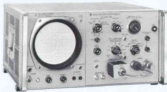
Fig. 2. Rise time converter is placed between STEP OUTPUT and SIGNAL IN connectors of -hp- TDR system, which consists of Model 1415A TDR Plug-in for Model 140A Oscilloscope.
