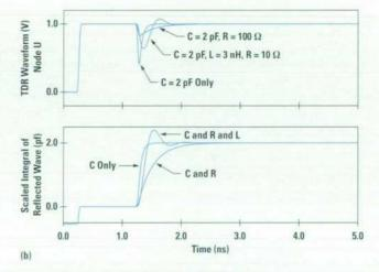
Fig. 12. L and R in series with a shunt capacitance do not affect the measurement of C.
