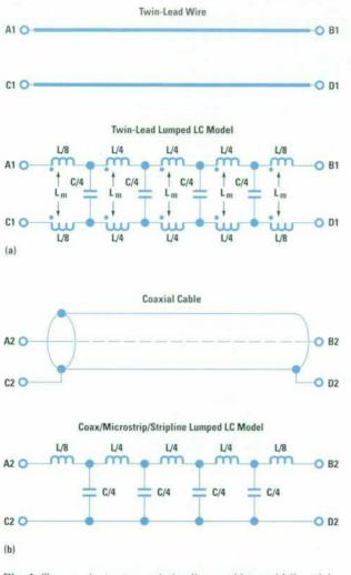
Fig. 1. Two-conductor transmission lines and lumped LC models.
