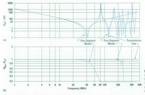
Fig. 3. (a) Magnitude of the input impedance  $Z_{\rm In}$  for the transmission line and models of Fig. 2. (b)  $|V_{\rm Out}/V_{\rm In}|$  for the transmission line and models of Fig. 2 (in the circuit at the bottom of Fig. 2).
