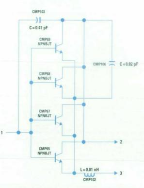
Fig. 13. HP Microwave Design System model for a full single cell.
