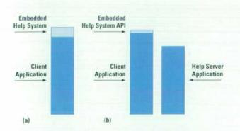
Fig. 1. Two different approaches to integrating online help into an application. (a) Client-side embedded implementation. This is the scheme used in CDE 1.0. (b) Server-side implementation of the help system. This was the implementation used in HP VUE 2.0.
