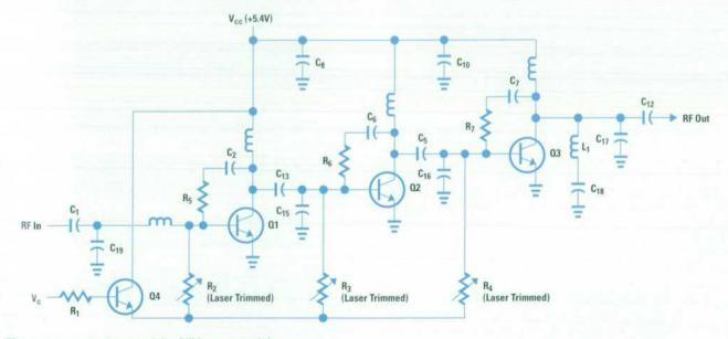
Fig. 3. Schematic diagram of the GSM power module.
