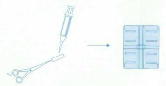
Fig. 6. Procedure for sample application (loading) onto a Zitex C-terminal sequencing membrane. sequenceable cycles. The high-sensitivity C-terminal sequence analysis is compatible with a great variety of samples encountered at these amount levels in research laboratories.
