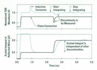
Fig. 14. Intermediate discontinuities do not affect the measurement as long as the discontinuity to be measured can be isolated on the TDR waveform.
