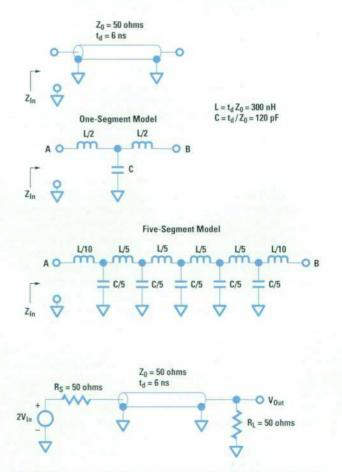
Fig. 2. Two LC models for a coaxial cable. The five-segment model is accurate over a wider range of frequencies than the one-segment model.
