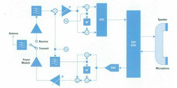
Fig. 1. Block diagram of a typical handheld digital telephone.
