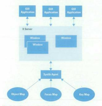
Fig. 2. Synlib test execution architecture.
