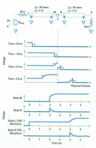
Fig. 11. A series capacitance between two transmission lines can be measured using the transmitted waveform (time-domain transmission or TDT) rather than TDR.
