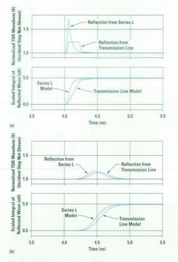
Fig. 9. (a) TDR waveforms from a SPICE simulation showing reflections from an ideal 4.88-nH inductor and an 80-ohm, 100-ps transmission line, both in a 50-ohm system. The final value of the integral of the reflected wave is the same for both. (b) Same as (a) for an incident step with a longer rise time. The agreement between the reflected waves for the single-inductor model and the transmission line is better. The final value of the integral of the reflected wave is unchanged.
