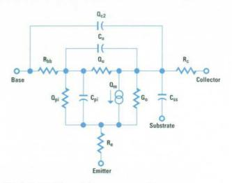
Fig. 9. Modified Gummel-Poon n-p-n ac model.
