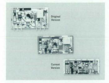
Fig. 2. GSM power module evolution.
