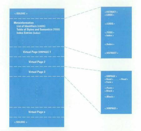
Fig. 7. The structure and elements of an SDL volume.
