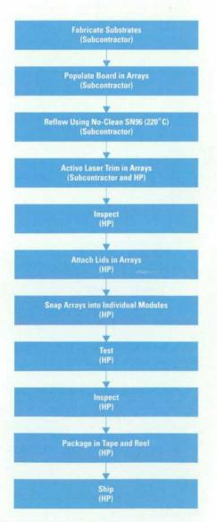
Fig. 5. Volume assembly process flow.
