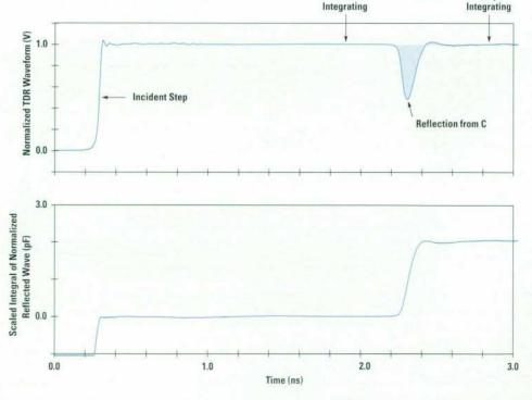
Fig. 6. (top) Measured TDR waveform from a 50-ohm microstrip trace with a discrete capacitor to ground at the middle of the trace. (bottom) The integral of the reflected waveform reveals that the capacitance is 2.0 pF.
