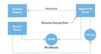
Fig. 1. Linkages for remote application execution.
