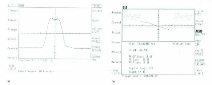
Fig. 10. Connecting the outputs of the HP 71910A to an HP 70703A high-speed oscilloscope enables the capture and display of much information from a radar signal. (a) A narrow 20-ns pulse. (b) An FM chirp.
