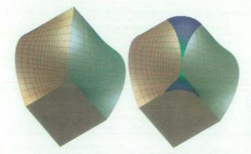
Fig. 8. If the primary surfaces have the same normal along the edge, the blend surface (blue) degenerates.
