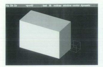
Fig. 3. The first step in the I-LOP (intelligent local operation) approach for a stretch (move face) operation in HP PE/Solid-Designer is the generation of the tool body, a four-sided prism in this case.
