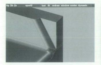
Fig. 16. The part of Fig. 13 changed by I-LOPs without the knowledge that there is a blended edge.
