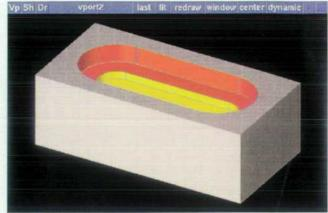
Fig. 11. Part with a countersunk pocket.
