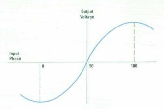
Fig. 24. Transfer function for a double-balanced mixer.
