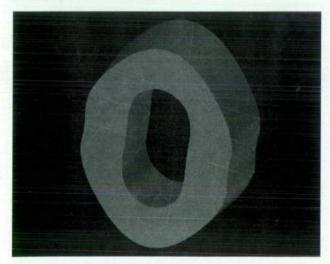
Fig. 7. Closed (periodic) surface created using lofting.
