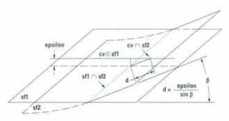
Fig. 2. A shallow intersection between the two surfaces sf1 and sf2 and the intersection with sf2 of a curve (cv) contained in sf1.
