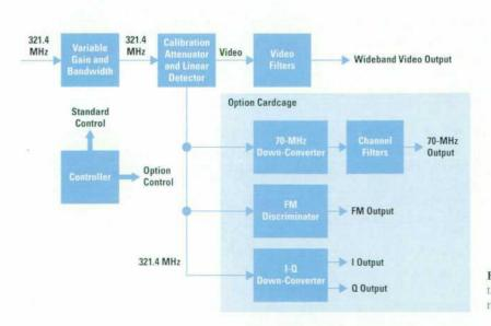
Fig. 4. The major functional blocks that make up the HP 70911A IF module. Fig. 4 shows the major functional blocks that make up the HP 70911A. The variable gain and bandwidth block includes a bandpass filter with bandwidth that varies from 10 to 100 MHz with DAC control. The filter is a five-pole synchronously tuned design. The gain consists of seven stages of step gains interspersed with the poles of the filter.
