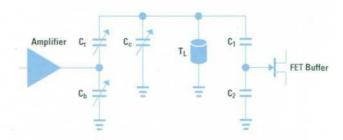
Fig. 9. 1-MHz-to-10-MHz bandwidth filter stage.
