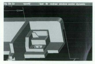
Fig. 15. The part of Fig. 13 with the new ramp angle (the ramp has been removed).
