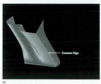
Fig. 10. (a) Illegal body with gaps between faces. (b) The system generates a common edge to eliminate gaps.
