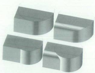
Fig. 10. Selecting the correct intersection point between a blend boundary and an adjacent edge also depends on the local surrounding geometry.
