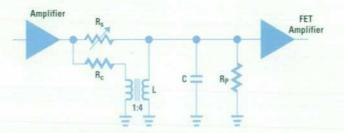
Fig. 5. Feed-forward amplitude compensated RLC tank circuit
