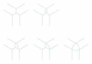
Fig. 19. Sequence of Euler operators used to create the face of Fig. 18.
