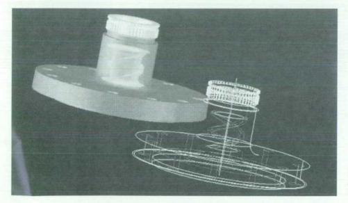
Fig. 11. Imported wire-body and the solid model constructed by HP PE/SolidDesigner.  Provides long-term neutral data storage and interpretability. Product data is an important asset of a manufacturing company. The product data should be retrievable and interpretable by any CAD or CIM system after a long period of time, say 10 years or more. This is a significant challenge.
