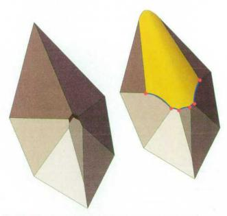
Fig. 14. Trimming a blend surface involves a number of curve/ surface intersections (red points) and surface/surface intersections (blue curves). Note how the faces marked dark red are "eaten up" by the blend face.
