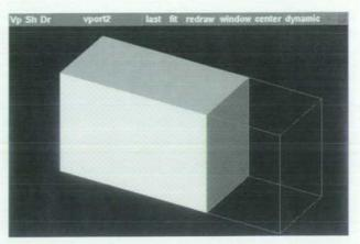
Fig. 4. The second step in stretching the box of Fig. 3 is to force the faces of the tool body to the final geometry, using a B-LOP (basic local operation).
