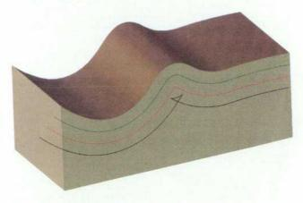
Fig. 7. When the blend radius is chosen too big, the blend boundary will have a cusp (red curve) or even be self-intersecting (black curve).
