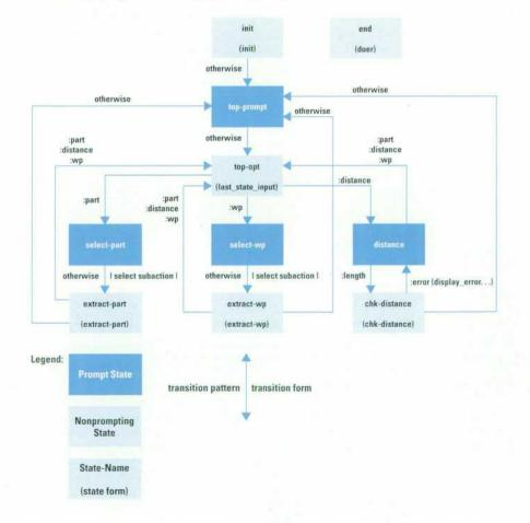
Fig. 10. State machine for the extrude command.
