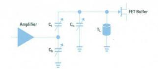
Fig. 8. Resonator with circuitry for bandwidth and center frequency tuning.
