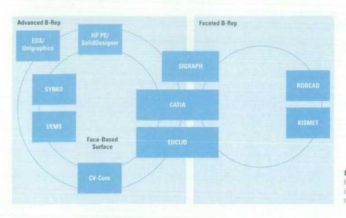
Fig. 14. Data exchange cycles between different CAD systems, including robot simulation systems, in the ProSTEP project.
