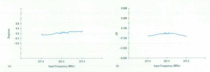
Fig. 30. (a) I-Q quadrature phase error. (b) I-Q amplitude imbalance.
