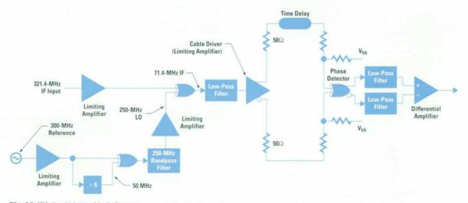
Fig. 26. FM discriminator block diagram.
