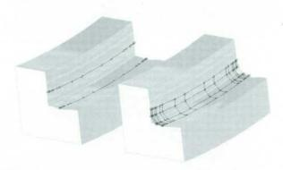
Fig. 13. Creating the geometry of a freeform blend surface: the control polygon of the blend boundaries (left) and the resulting blend surface (right).
