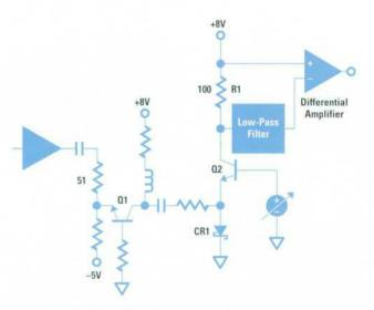
Fig. 18. Linear detector circuit.
