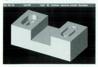
Fig. 10. Part with one compound pocket and a boss inside a pocket.
