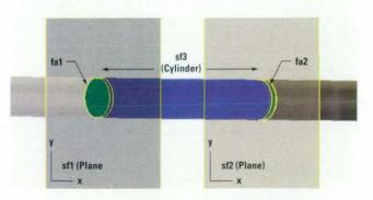
Fig. 8. An example of the relationship between topology and geometry. Faces and edges bound or trim their geometries, which consist of infinite curves and surfaces.
