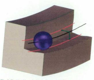
Fig. 6. The blend boundaries (red) are created by mapping the spine (black) onto the primary surfaces.
