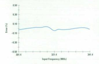
Fig. 27. Discriminator linearity error (percent of full scale).
