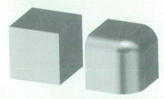
Fig. 4. Three cylindrical blends with different radii connected by a freeform vertex region.
