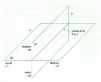
Fig. 10. Surfaces split space into halves called half spaces (inside and outside along surface normals). Each piece of a split surface can be classified as belonging to a half space with respect to the other surface.
