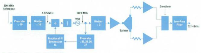
Fig. 29. Block diagram of the 321.4-MHz LO.
