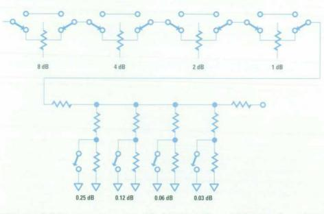
of fixed switchable attenuator sections (Fig. 14). The 1-dB through 8-dB attenuator stages are pi attenuators made with surface mount thick-film resistors. The 0.25-dB through 0.03-dB attenuator stages could not be designed as pi attenuators because the resistance values required for these very low attenuation values would not be achievable at 321.4 MHz.
