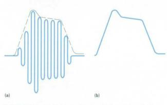
Fig. 17. (a) Input to the linear detector. (b) Output from the linear detector after the carrier is stripped off.
