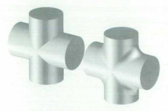
Fig. 24. Another example of two adjacent surfaces that have the same normal at an endpoint of an edge to be blended. The trimming part of the algorithm is not needed.
