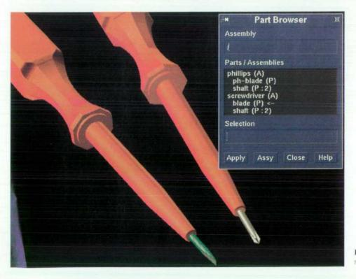
Fig. 4. Two assemblies with shared parts.
