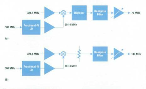
Fig. 21. Simplified block diagram of the output options for direct connection to commercial demodulators. (a) 70-MHz IF output. (b) 140-MHz IF output.
