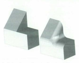
Fig. 21. A transition curve (lower edge of the vertex region) is also inserted when two adjacent blend boundaries around a vertex region don't intersect.
