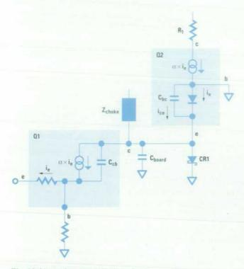
Fig. 19. Linear detector equivalent circuit.
