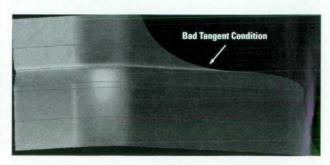
Fig. 17. Positioning too many profiles over too short a distance results in a wavy surface.
