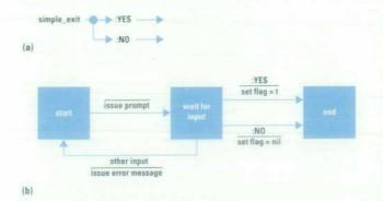
Fig. 2. (a) Simplified syntax of the exit command. (b) State transition diagram for the exit command.
