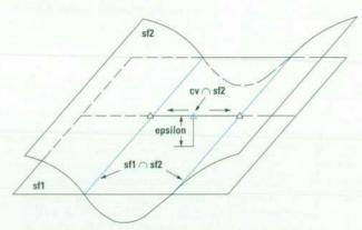
Fig. 4. A geometric configuration in which the intersection between sf1 and sf2 yields two intersection tracks (colored lines) but the intersection of the curve contained in sf1 with sf2 gives one intersection point (colored triangle) which is farther than the resolution away from the tracks.
