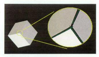
Fig. 1. In solid models edges seem to be exactly on their adjacent faces and meet exactly at their common vertices. In reality, because of the limited floating-point accuracy of a computer, on the microscopic level there are gaps and holes everywhere.
