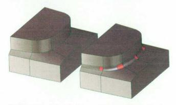
Fig. 22. Additional faces (red) are inserted where adjacent blends are tangentially connected.
