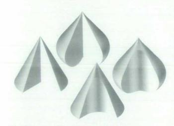
Fig. 23. When material is added by blending an edge, an apex might move from the boundary to the interior of a face.
