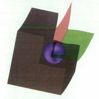
Fig. 5. The center of the rolling ball moves on the intersection curve between the two offset surfaces.
