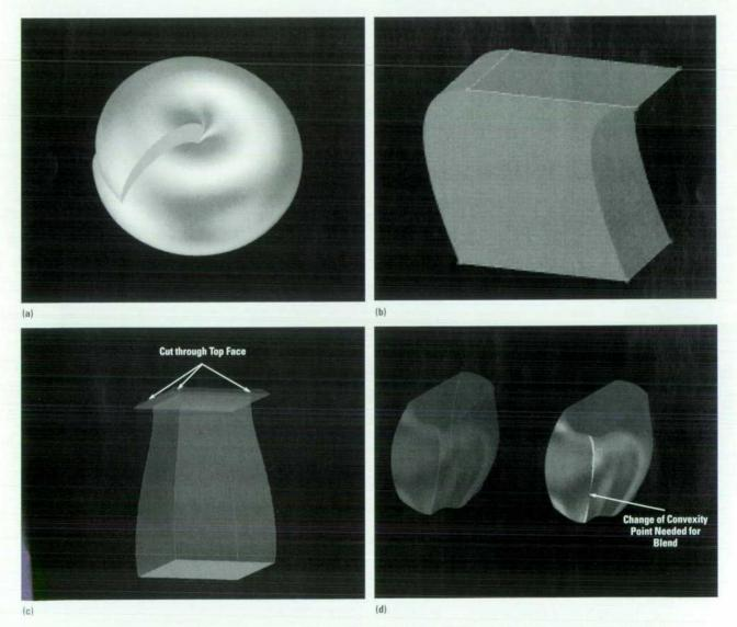
Fig. 14. HP PE/SolidDesigner checks for various properties that solid bodies shouldn't have. (a) Self-intersecting body. (b) Vanishing normals or derivatives. (c) Intersection with the top or bottom face. (d) Change of convexity at an edge.
