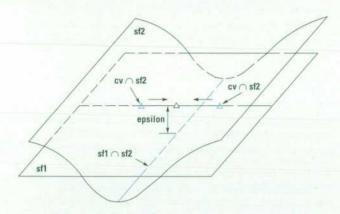
Fig. 3. A geometric configuration in which the intersection between sf1 and sf2 yields one intersection track (colored line) but the intersection of the curve contained in sf1 with sf2 gives two intersection points (colored triangles) which are farther than the resolution away from the track. into a single point (black triangle) which is closer than the resolution to the intersection track (colored line).
