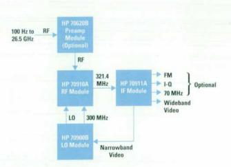
Fig. 2. A simplified block diagram of the main components of the HP 71910 Option 011 receiver.
