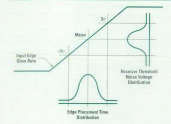
Fig. 3. Jitter, as it occurs in clock buffers, is generally the result of noise in the power environment (return currents, image currents, etc.) modulating the switching threshold of the buffer.
