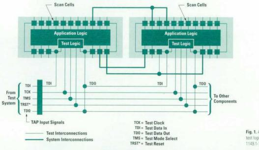
Fig. 1. A simplified block diagram of the test logic defined in ANSI/IEEE Standard 1149.1-1990 surrounding application logic.
