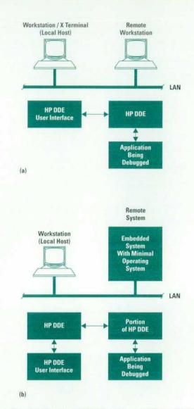
Fig. 4. Two possible remote HP DDE sessions. (a) Most of HP DDE and the application being debugged are run on a remote system and the HP DDE user interface is run from an X terminal. (b) Most of HP DDE is run on a local host and a portion of HP DDE and the application are run on a remote system.
