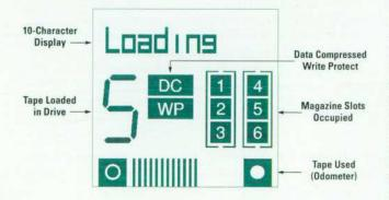
Fig. 6. Liquid crystal display layout.
