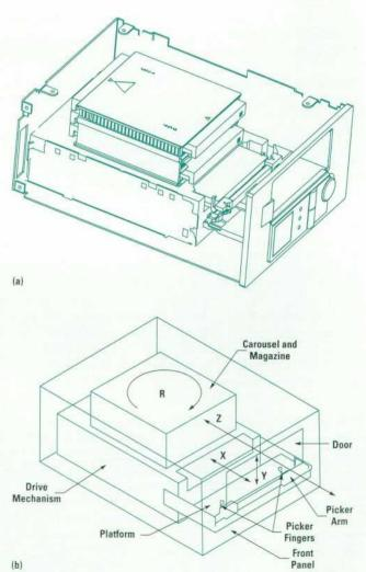
Fig. 3. (a) Interior layout of the HP C1553A autoloader. (b) Motions of the cartridge changing mechanism.
