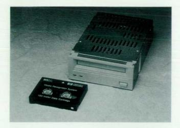
Fig. 2. The HP C1533A DDS-2 tape drive has a native-mode data transfer rate of 510 kbytes/s, 40% faster than other designs. It records on high-capacity 4-Gbyte DDS-2 cartridges or on earlier DDS media.
