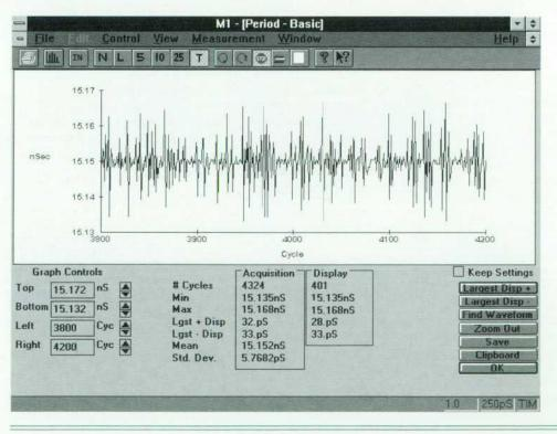
Fig. 2. There are a number of metrics of jitter. This measurement shows the cycle-to-cycle variation in the period of a 66-MHz clock. This was made using the Amherst Systems Associates M1 time interval measurement software, which analyzes digitized waveform data from an HP 54720D oscilloscope for jitter in a variety of ways.
