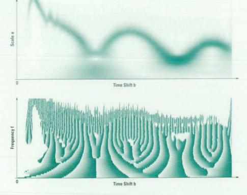
Fig. 23. Magnitude of the wavelet transform of transmitter turn-on
