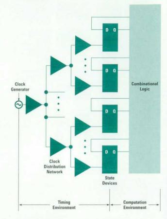
Fig. 1. State architecture model. Any synchronous digital system can be decomposed into a timing environment and a compute environment. The design issues specific to the timing environment are becoming critical in PC and workstation designs.
