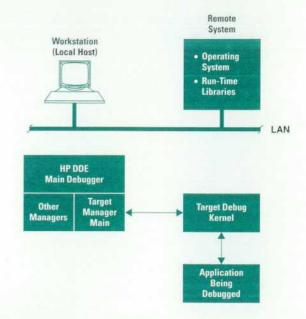
Fig. 6. Remote debugging session showing the distribution of the target manager software.
