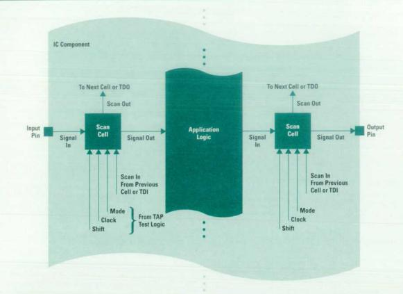
Fig. 2. The location of scan cells in relation chip I/O pins and the application logic. The mode, clock and shift signals are derived from the TAP input signals TMS, TCK, and TRST\* respectively. The first scan-in signal and the last scan-out signal correspond to TDI and TDO respectively.
