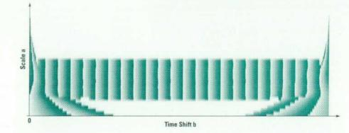
Fig. 12. Phase of the wavelet transform of a constant-frequency sinusoid.
