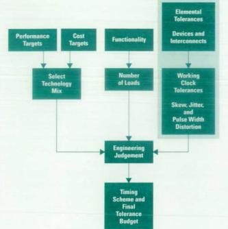
Fig. 1. Timing environment design process. Design-specific and/or unrated parametric information must be incorporated into the engineering decision making process from the outset.
