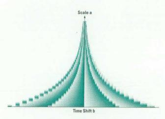
Fig. 2. Phase of the wavelet transform of a delta function.
