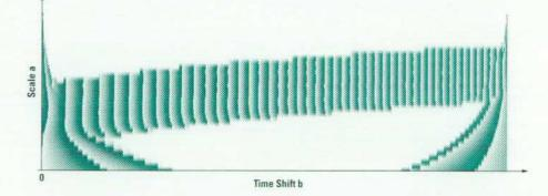
Fig. 15. Phase of the wavelet transform of a sinusoid with linearly increasing frequency.
