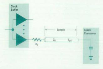
Fig. 4. Most of the clock nets in our design can be viewed as simple series-terminated transmission lines driving single capacitive loads.
