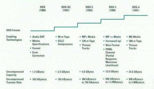
Fig. 1. Evolution of the DDS tape format.
