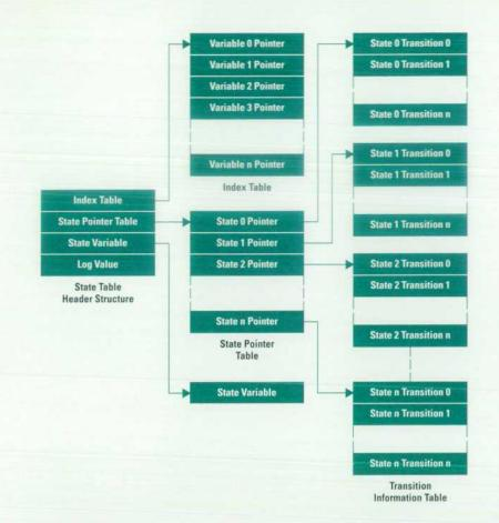
Fig. 2. State table data structures.
