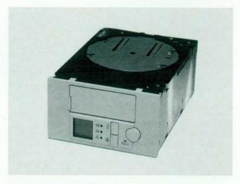
Fig. 1. The HP C1553A DDS-2 digital audio tape autoloader contains a DDS-2 tape drive and a cartridge changing mechanism that selects one of six cartridges from a magazine and loads it into the drive. Cartridges are changed automatically under software control.
