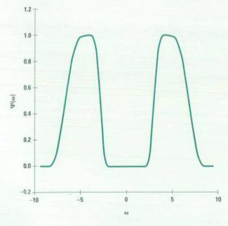
Fig. 4. Fourier transform of the Meyer wavelet.
