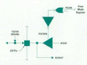
TESTDEN = 0 when TESTER DRIVING Is Sending Input to I/O Pin = 1 when BUSIN Is Sending Output to I/O Pin
