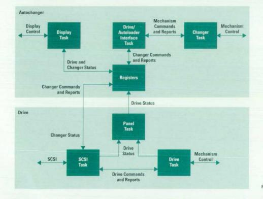
Fig. 1. Autoloader firmware architecture
