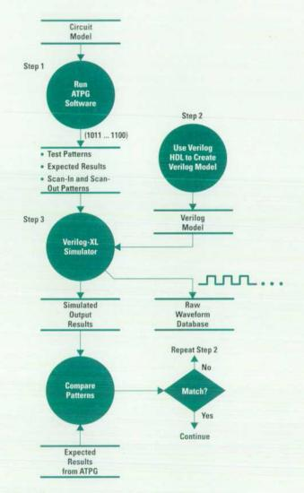
Fig. 1. The steps used to create a raw waveform data base.
