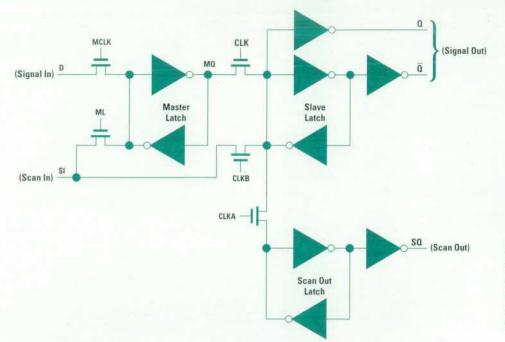
**Fig. 2.** Scannable flip-flop. This is a portion of our implementation of a scan cell. The MCLK, ML, CLKA, and CLKB signals are controlled by the TAP test logic and are derived from the TAP input signals TMS, TRST\*, and TCK.
