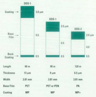
**Fig. 3.** DDS tape types. MP = metal particle. PET = polyethylene terathalate. PEN = polyethylene naphtalate. PA = polyamide.
