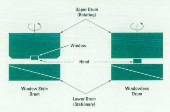
Fig. 8. Two styles of drums with gaps to bleed off excess air between the drum and the tape. In each case, four heads are spaced evenly around the drum, but only the one nearest the observer is shown in this drawing. The diagonal line on the lower drum is the path of the lower edge of the tape in this helical scan system. the tape drive, but many are dictated by the system using the tape drive. The major performance factors, along with the corresponding controlling functions, are listed below.
