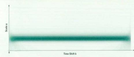
Fig. 11. Magnitude of the wavelet transform of a constant-frequency sinusoid.
