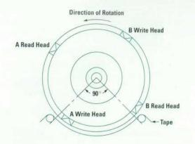
Fig. 4. The DDS tape drive has four heads mounted on a rotating drum. Only one head at a time is in contact with the media.
