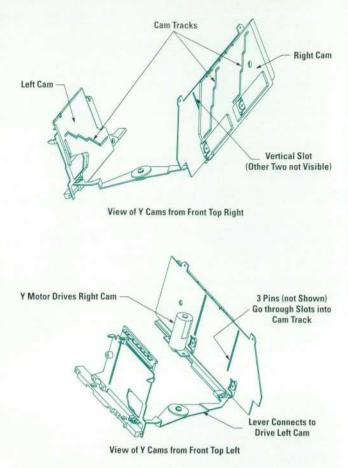
Fig. 4. Y-motion cam design. (a) View of the Y cams from the front top right. (b) View of the Y cams from the front top left.
