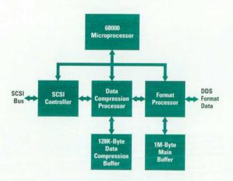
Fig. 9. Block diagram of the HP C1533A tape drive controller.
