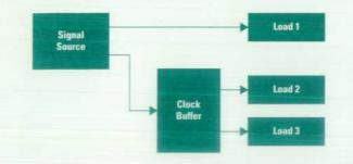
Fig. 7. The margin available at a specific load in a system can be examined by driving that load from a two-channel signal source and carefully adjusting the relative phase of the channels until unreliable switching is detected.
