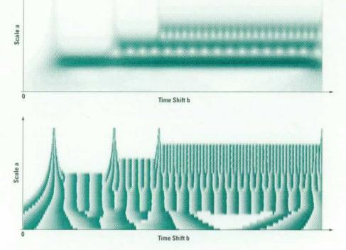
Fig. 20. Magnitude of the wavelet transform of three sinusoids with different starting times.
