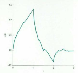
Fig. 8. The Daubechies scaling function for N = 2.
