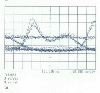
Fig. 9. (a) Conventional eye diagram of a low-level signal. (b) Eyeline diagram of a low-level signal with eye filtering applied.
