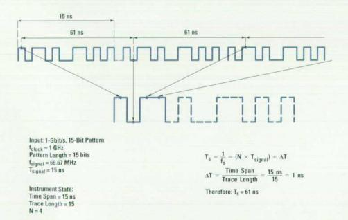
Fig. 8. Harmonic repetitive sampling of a PRBS waveform to generate an eyeline diagram. Thus, every fourth cycle of the pattern, the sampling point moves forward 1 ns, and after sixty cycles of the pattern waveform, one complete trace of the pattern is displayed.
