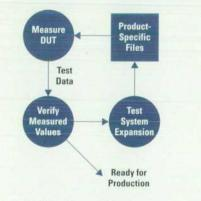
Fig. 8. Data-driven initial product testing.
