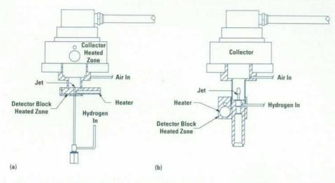
Condensation forms from the combustion of hydrogen and air when the detector block temperature is below 100°C. Table II is a comparison of the GC and SFC detectors.
