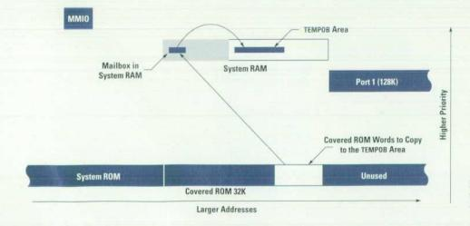
Fig. 5. Copy-to-TEMPOB configuration for HP 48S/SX covered ROM words.
