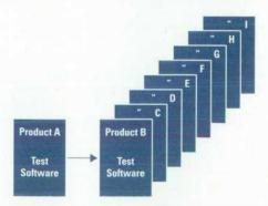
Fig. 2. Product-specific test software requires introduction or reworking of the software for each new product.
