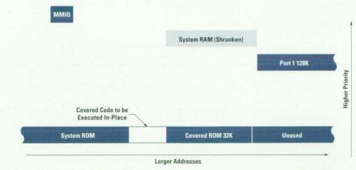
Fig. 3. Execute-in-place configuration for HP 48S/SX covered code.
