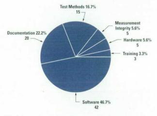
Fig. 1. Average proportions of time spent developing various manufacturing resources for a group of electrical test processes. Software dominates because the division is moving towards completely automated testing.
