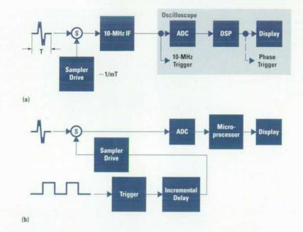
Fig. 5. Simplified architectural comparison of the eye diagram analyzer (a) and a conventional sampling oscilloscope (b).
