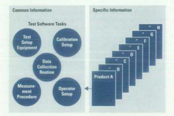
Fig. 3. In data-driven software, product-specific information is removed from the test software and stored in files. The software doesn't have to be changed to test a new product within the product classification.
