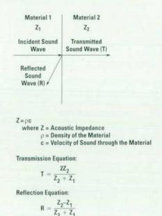
Fig. 1. Sound waves traveling between two materials.
