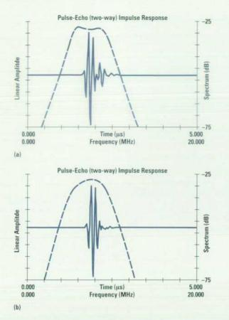
Fig. 14. (a) Pulse and spectrum of the modeled HP 21258A 7.5-MHz transducer. (b) Pulse and spectrum of the modeled HP 21258B 7.5-MHz transducer.
