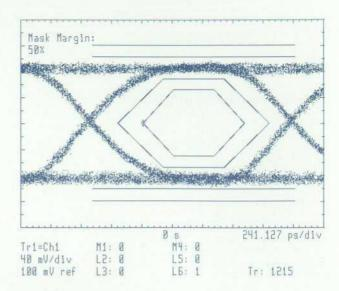
Fig. 12. Eye mask measurement.
