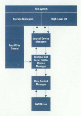
Fig. 1. Original driver architecture.
