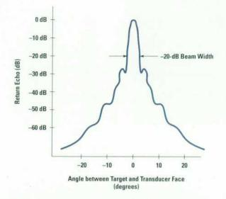
Fig. 8. Typical lateral beam plot at some distance from the transducer, showing beam width measurement.
