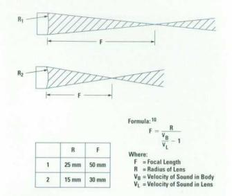
Fig. 10. Influence of lens radius on focal point and elevation beam width.
