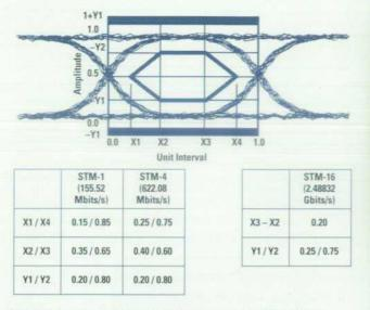
Fig. 3. Laser transmitter eye diagram masks for SONET/SDH transmission systems.
