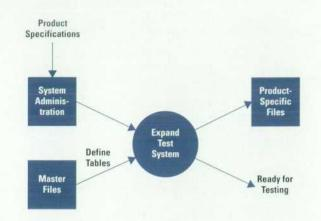
Fig. 6. Data-driven test system expansion.
