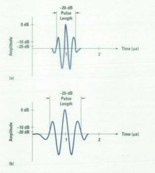
Fig. 11. Comparison of ultrasound pulses from transducers operating at different frequencies. (a) 7.5-MHz pulse. (b) 4.5-MHz pulse.
