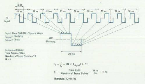
Fig. 7. Harmonic repetitive sampling of a waveform.
