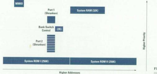
Fig. 12. HP 48G standard configuration.
