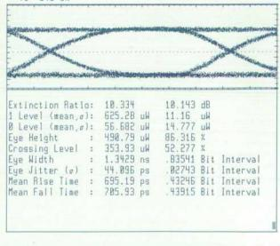
Fig. 11. Table of eye diagram parametric measurements.
