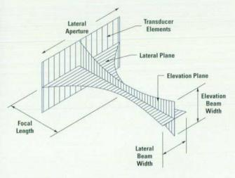
Fig. 7. Focused beam, showing elevation and lateral planes.
