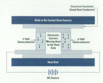
Fig. 2. Thermoelectric (Peltier) cooler.
