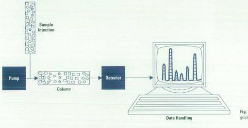
Fig. 1. Basic components of a chromatographic system.
