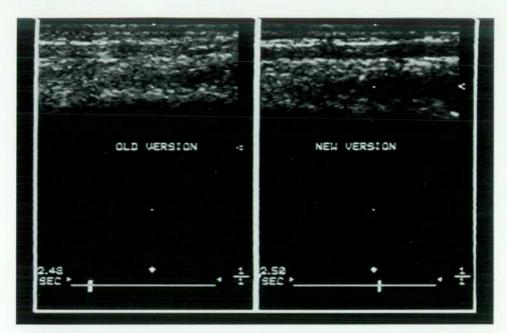
Fig. 16. 2D images of the radial artery in the arm. (left) HP 21258A transducer. (right) HP 21258B transducer.
