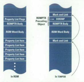
**Fig. 6.** Comparing the structure of a ROM word as resident in ROM and when copied to TEMPOB using covered technology.
