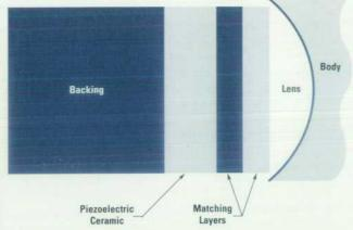
Fig. 6. Enlarged side view of one element of an ultrasound transducer.
