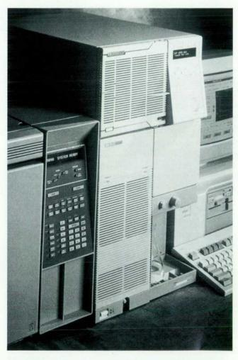
Fig. 1. HP G1205A supercritical fluid chromatography system.
