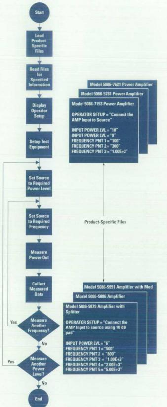
Fig. 4. Data-driven amplifier power test.
