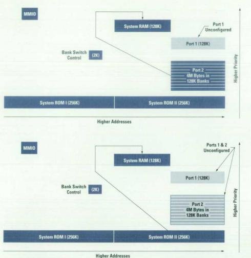
Fig. 8. HP 48GX configuration for copying an object from a bank of port 2 to TEMPOB.
