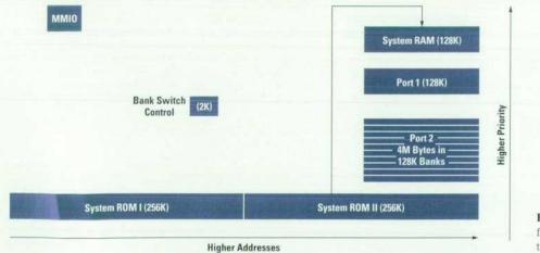
Fig. 10. HP 48GX configuration for copying an object to TEMPOB through a mailbox.
