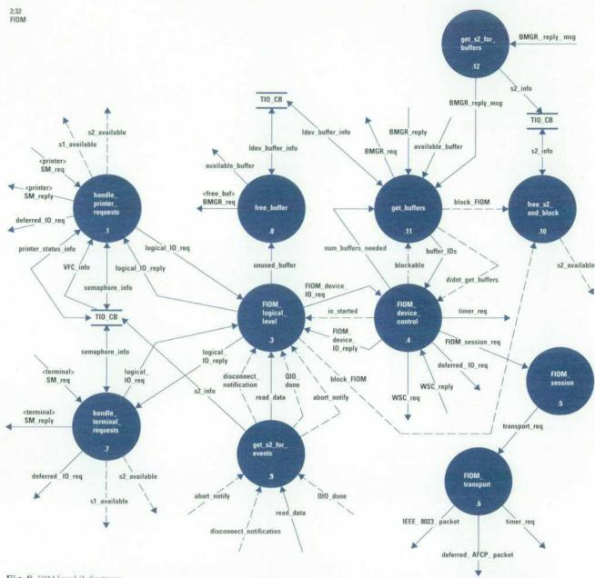
Fig. 8. FIOM level 2 diagram.
