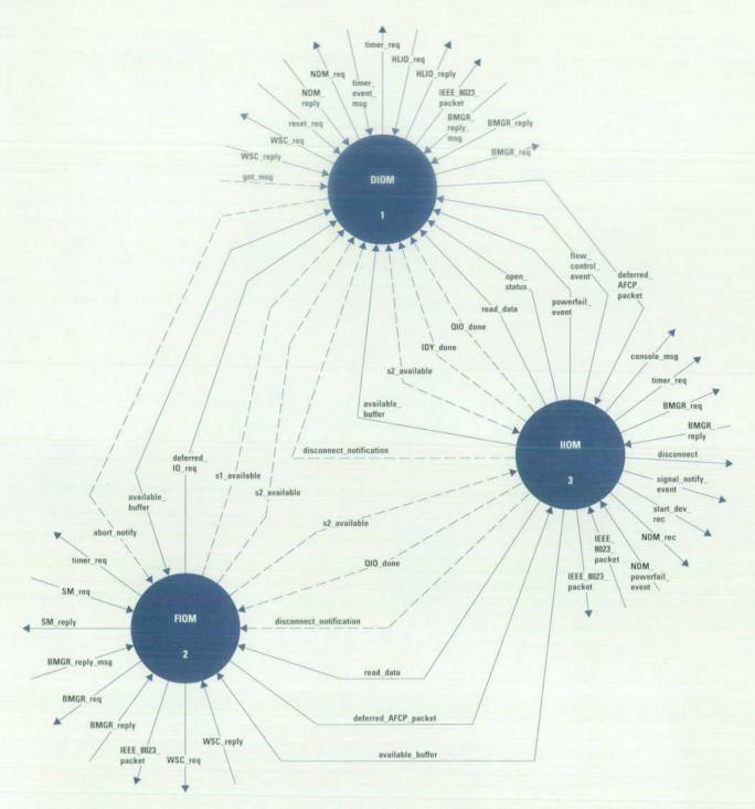
Fig. 7. Driver level 1 diagram showing the three major modules: the fast I/O manager FIOM, the deferred I/O manager DIOM, and the inbound I/O manager IIOM.
