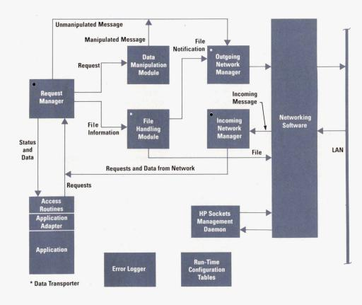
Fig. 4. HP Sockets run-time architecture.
