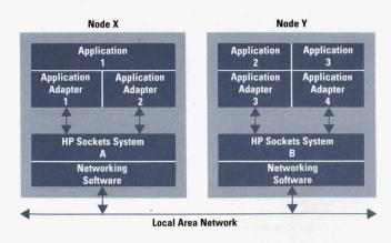
Fig. 5. Application integration with HP Sockets.
