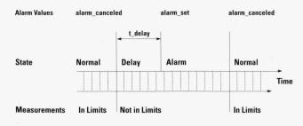
Fig. 1. Measurements, states, and alarm values.
