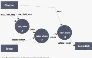
Fig. 1. Composition diagram for the alarm system
