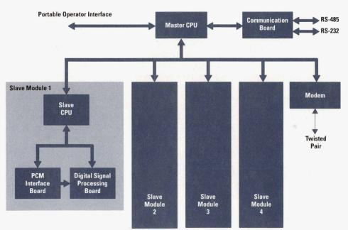
Fig. 3. Peripheral unit architecture.
