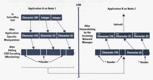
**Fig. 12.** A simplified illustration of the data manipulation, marshaling, and unmarshaling of data in the HP Sockets domain.
