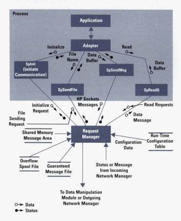
**Fig. 7**. Structure chart showing the communication data flows between the request manager and some of the HP Sockets access routines. Since the routine was called with wait, the SpSendMsg call will not return to the calling routine until it either receives a status value back from the request manager or times out.
