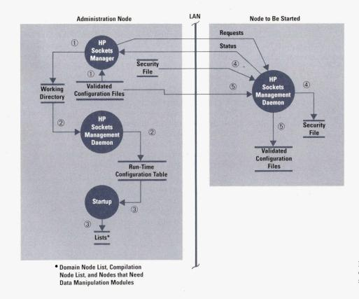
**Fig. 10**. Some of the processes and data flows involved in HP Sockets startup.
