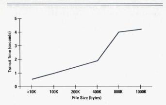
Fig. 2. HP Sockets file transit time as a function of file size using an HP 9000 Series 370.
