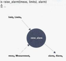
Fig. 6. Data flow diagram of the  $\mathsf{raise\_alarm}$  process with the correct data flows.
