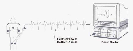
**Fig. 2.** Setup for making ECG measurements, showing the stream of voltage signals from one of the ECG leads.
