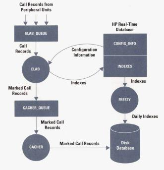
Fig. 4. Simplified block diagram of the elaboration software.
