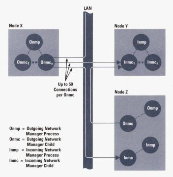
Fig. 8. Outgoing and incoming network manager processes and their connections.
