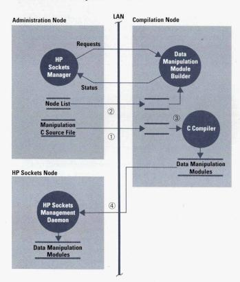
**Fig. 11.** Activities taking place between the administration node and a compilation node during startup and the creation of data manipulation modules.
