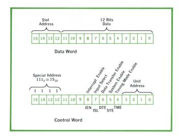
**Fig. 3.** Digital words used by Multiprogrammer. Each channel is addressed by bits 12–15 in data word. Remaining bits carry data. To control Extenders, control word with special address in bits 12–15 precedes data word. Bits 0–3 in control word select Extender to receive data words that follow.
