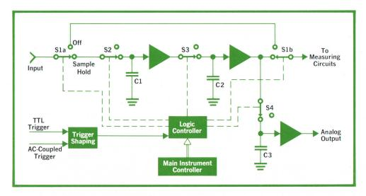
Fig. 6. Sample-and-hold retains instantaneous value of input level on capacitor C1 when switch S2 opens. Switch S3 opens 2 ms later, giving time for C2 to charge to same voltage as C1. Instrument measures voltage retained on C2.
