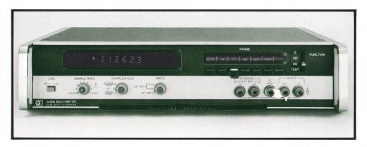
Fig. 1. Model 3490A Digital Multimeter measures dc volts, ac volts and resistance with 10 ppm resolution. Model shown here has Ratio and Sample-and-Hold options installed. Easy-to-decipher range and function control brings into view only those ranges needed for function selected. Depressing appropriate tab selects range desired. Slideout instruction card includes operator instructions for using Multimeter to test itself.
