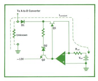
**Fig. 6.** Ohms converter has amplifier that adjusts series regulator Q1 impedance to maintain current through R<sub>ref</sub>, and thus through unknown, constant. Voltage across unknown therefore is proportional to unknown's resistance.
