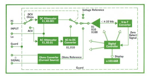
Fig. 3. Simplified block diagram of Model 3490A Multimeter in its basic configuration. Input signals go directly into guard (metal shield that electrically isolates circuits from power line to avoid ground loops and give 140-dB suppression of common-mode signals). Digital information to and from external equipment is coupled into and out of guard by light-coupled isolators (not shown).
