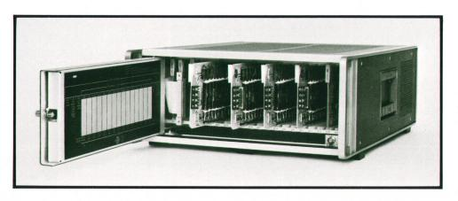
Fig. 4. Model 6940A accepts up to 15 input and output cards (four shown here partially inserted) in any combination. Cards are easily added, removed, or interchanged to modify capabilities of data acquisition and control system.
