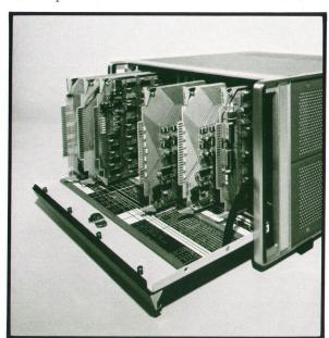
**Fig. 1.** Model 2440A Analog-Digital Interface is designed to serve as the interface between a computer and the sensors monitoring a physical process. It's configured for a variety of data acquisition and control applications by plugging appropriate modules into a combining case.
