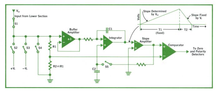
**Fig. 4.** Analog-to-digital converter in new Multimeter consists of voltage-to-time converter, shown here, and digital accumulator shown in Fig 5. Voltage-to-time converter generates time interval (T2) proportional to input voltage (V<sub>in</sub>).
