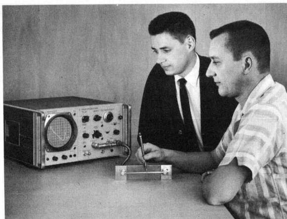
Fig. 1. Time domain reflectometer setup using -hp- Model 1415A plug-in unit with -hp- Model 140A Oscilloscope. Plug-in unit generates a fast step which is fed to external circuit. Energy reflected by discontinuities and impedance changes in external circuit returns to plug-in and is displayed on oscilloscope, permitting magnitude, sign and physical location of discontinuity to be read from scope face.
