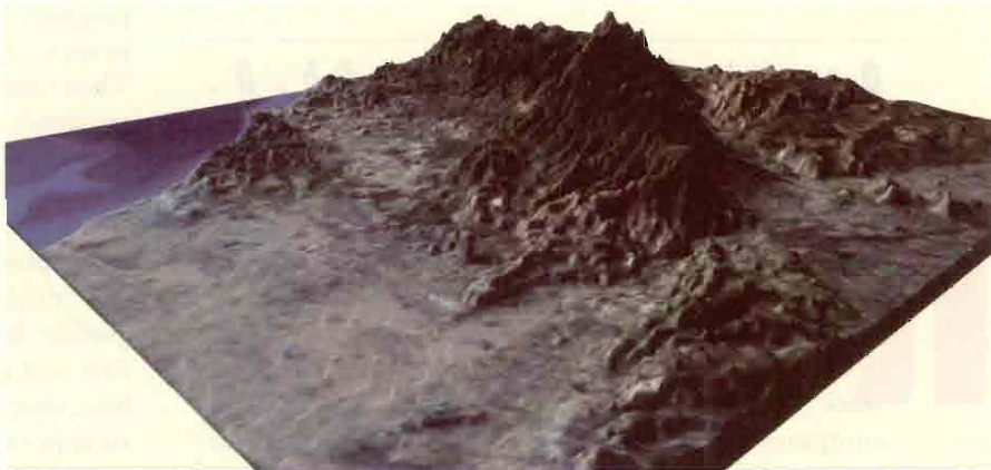
Figure 2. Object graphics 3D visualization of the image data in Figure 1 "draped" over a topographic terrain model.
