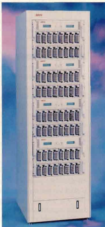
CSI selected six separate MTI 9300 RAID Level 5 Arrays each containing seven 4.29GB drives for a total of 180GB.
