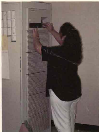
The HP 120T jukebox, with robotic picker, provides the BIA the means to store the one million and growing lease record documents.
