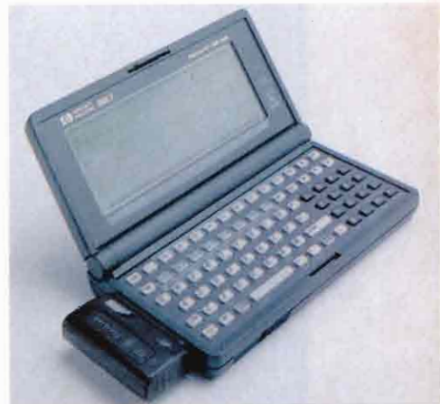
HP's PalmVue System uses a "doctored" HP 200LX palmtop to receive wireless transmissions of patient data.
