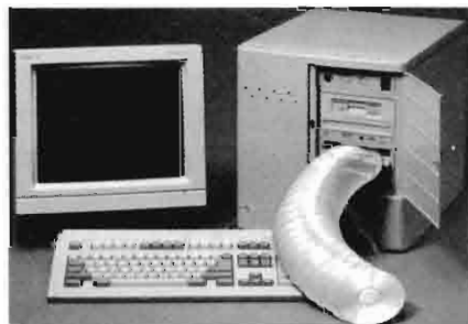
The CD-R CUBE creates CD-ROM disks from files or scanned images.
