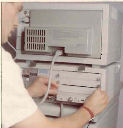
Don't open the cabinet: Just remove the backplane plates.
