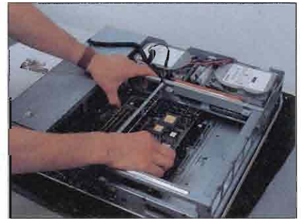
The board comes up easily after loosening the screws.
