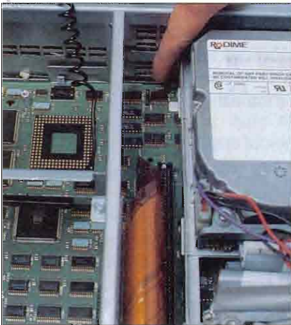
You need to move this jumper over so the 68040 can be used.
