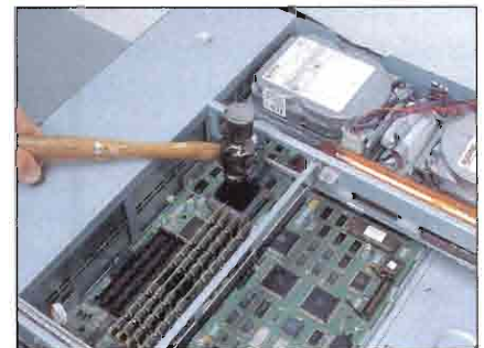
Socket for 68040 processor. Note empty crystal socket right next to the 68040 socket.
