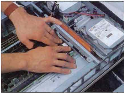
Gently pry the old chip loose and carefully insert the new one.
