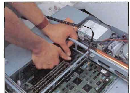
Press the 68040 chip in the socket firmly, but gently. (A hammer would be overkill.)
