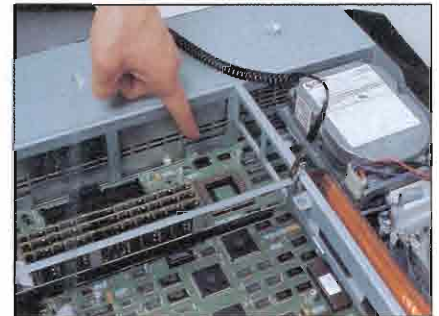
Socket for 68040 processor. Note empty crystal socket right next to the 68040 socket.
