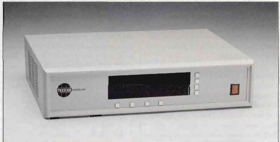
The RGB/Videolink 1600U scan converter transforms high-resolution computer graphics to television format in real time.
