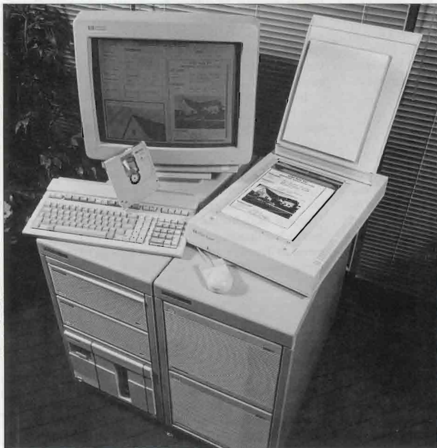
Hewlett-Packard's Advanced Image Management System (AIMS) lets users convert paper-based information into digital form to make the tasks of storing, retrieving, filing and manipulating information more efficient.
