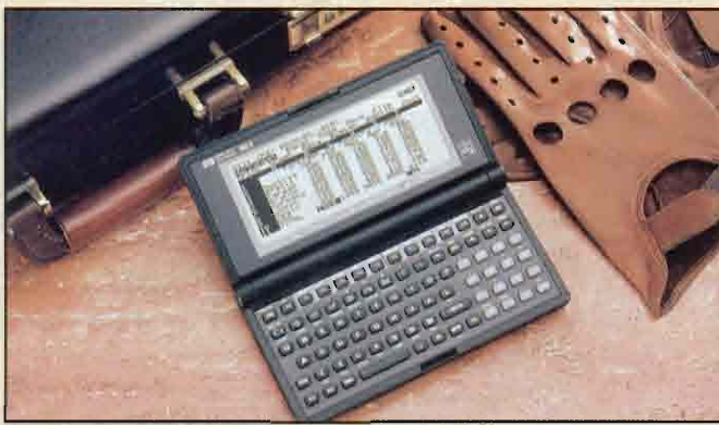
HP's 95LX palmtop combines HP calculator technology, DOS compatibility and the Lotus 1-2-3 spreadsheet.
