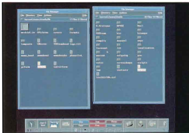
Figure 2: The File Manager provides a graphical means of navigating through your local UNIX file system and remote systems.
