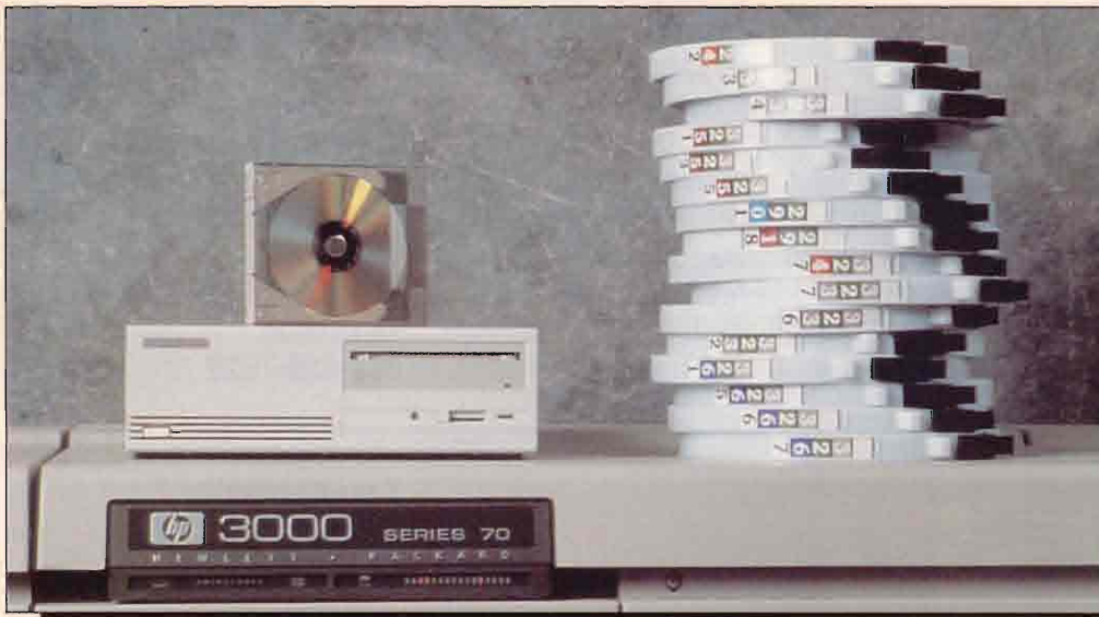
HP LaserRELEASE, a new program for distributing operating system and subsystem software for the HP 3000, uses CD-ROM instead of magnetic tape as the software-distribution media.
