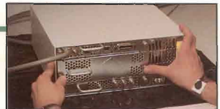
6a. When replacing the rear cover, make sure the connector pins mate properly with the connectors on the rear cover. You'll only get one chance.
