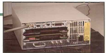
2a. With the cover off, you can see clearly the memory and CPU boards. You'll be hunting for the CPU board.
