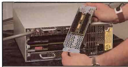
1a. Exercise care when removing the CPU/memory cover. You don't want to damage the connectors on the cover.
