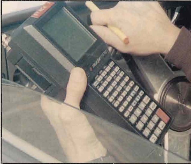
The Telxon 750 Radio Frequency Handheld Terminal unit (left) is used in Virginia International Terminal's Yard Management System to store location, size, weight and ultimate destination of each container (right).
