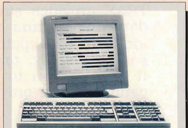
The HP 700/32 display terminal is for system users who require ANSI and DEC VT320 compatibility.
