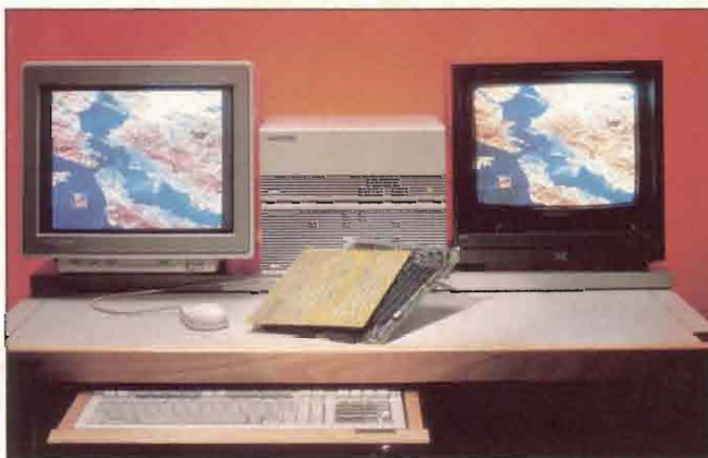
This picture shows the video out boards in front of the Series 300. The image on the screen is satellite information taken from the GOES satellite. The image on the left is the 1280 x 1024 computer output. The image on the right is the NTSC video out.
