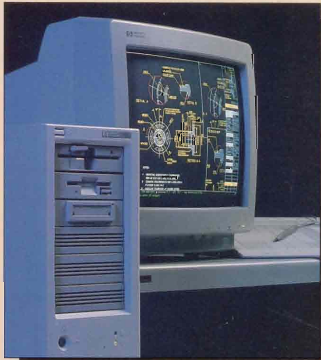
The ME10d is a software package for mechanical design and drafting and is full function DOS version of HP's UNIX system software.
