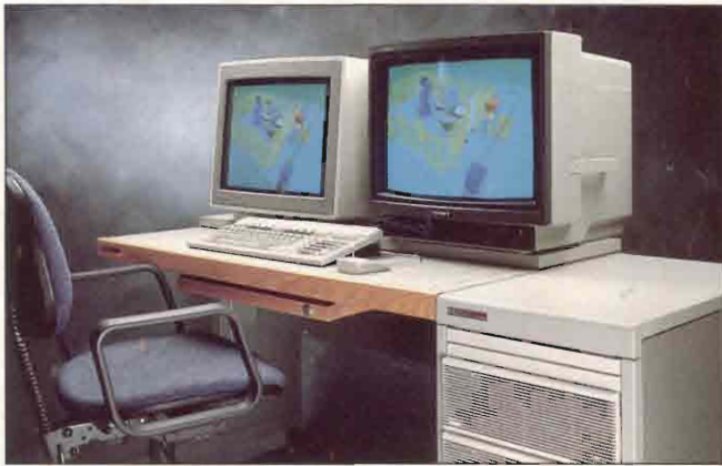
Shown is a Series 300 TurboSRX running software from Deneb Robotics and outputting the results to a standard Sony NTSC monitor using the Video/300 interface card.
