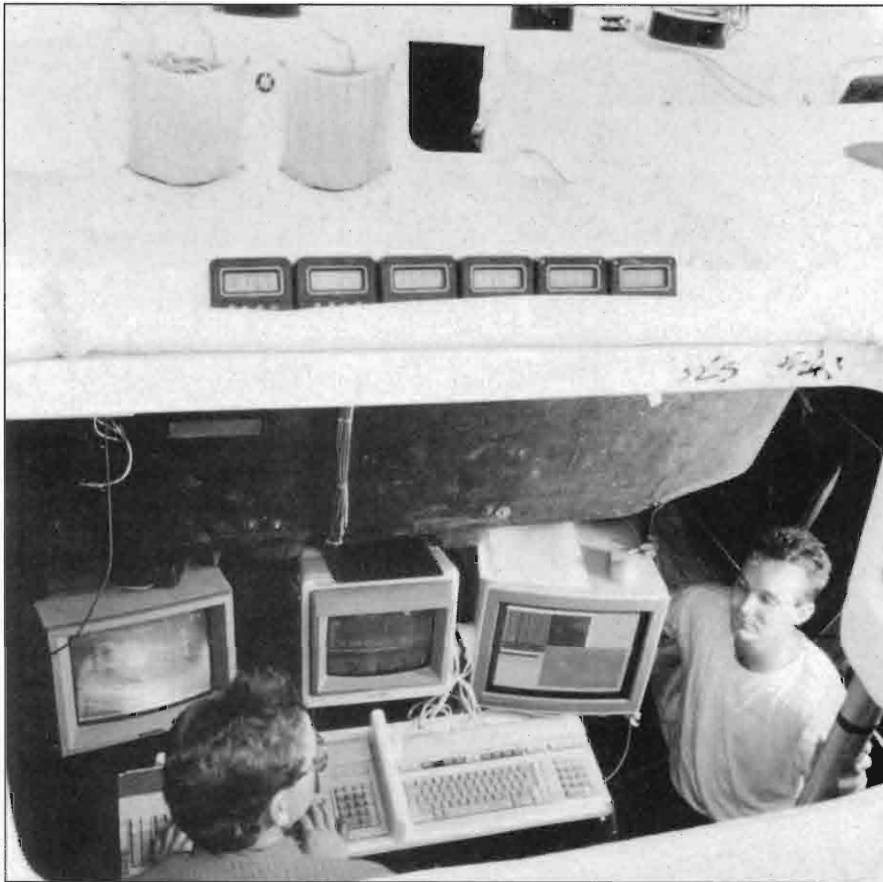
Three HP computer systems filled the cockpit of the "New Zealand." The computers were used to monitor and display information on boat performance, sail shapes, stress on the mast and rigging and for tactical navigation.
