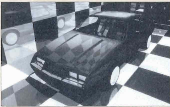
Ray tracing allows you to produce realistic highlights and reflections. Data to produce this image courtesy of Chrysler Corporation.
