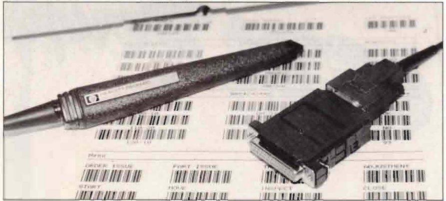
Minerva's Interface converts SmartWand output into RS-232C signal levels.
