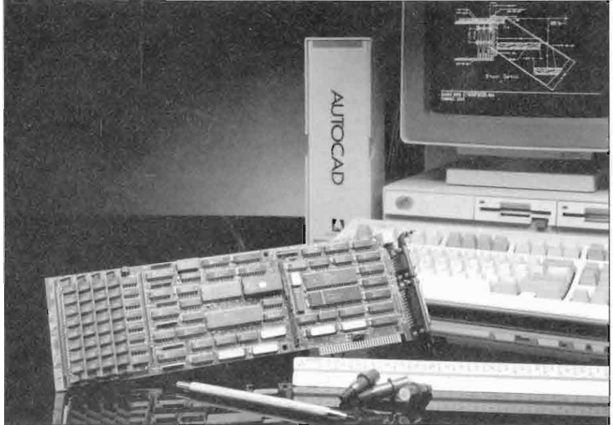
The SELERIS PC plugs into an open expansion slot inside any PC XT/AT or compatible computer, appearing as a standard serial communications port.
