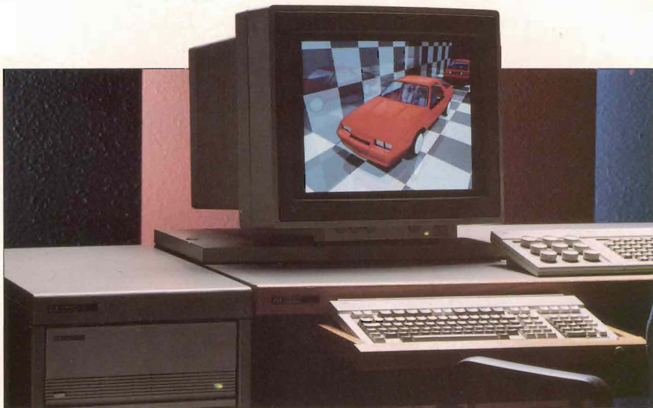
The new 350/835 TurboSRX workstation features Ray Tracing, a method used to produce very realistic highlights, reflections and transmittance effects.
