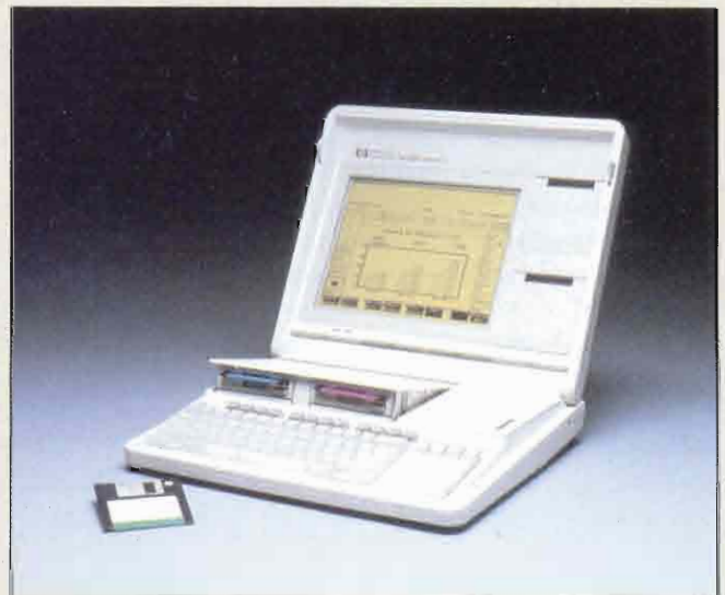
HP's Vectra CS personal computer is the industry's first portable to be equipped with a Hayes AutoSync 2400 bps modem.
