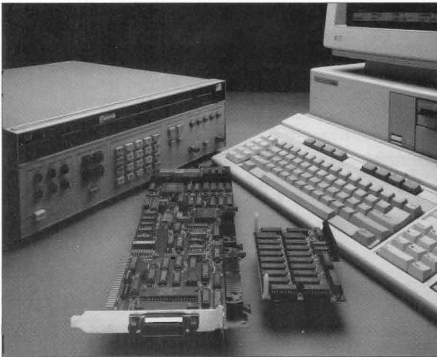
HP's Viper board and accompanying "piggyback board" for a total of 4 MB combined RAM/ROM.
