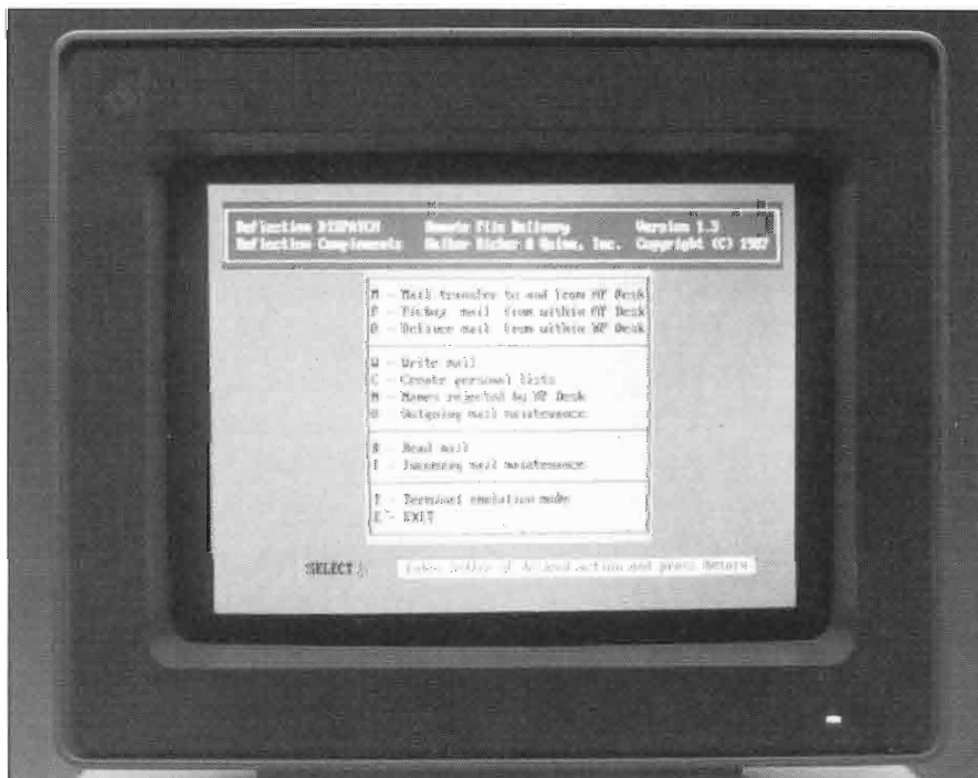
Using Dispatch, PC users connected with Reflection can read and compose HPDesk messages while offline.
