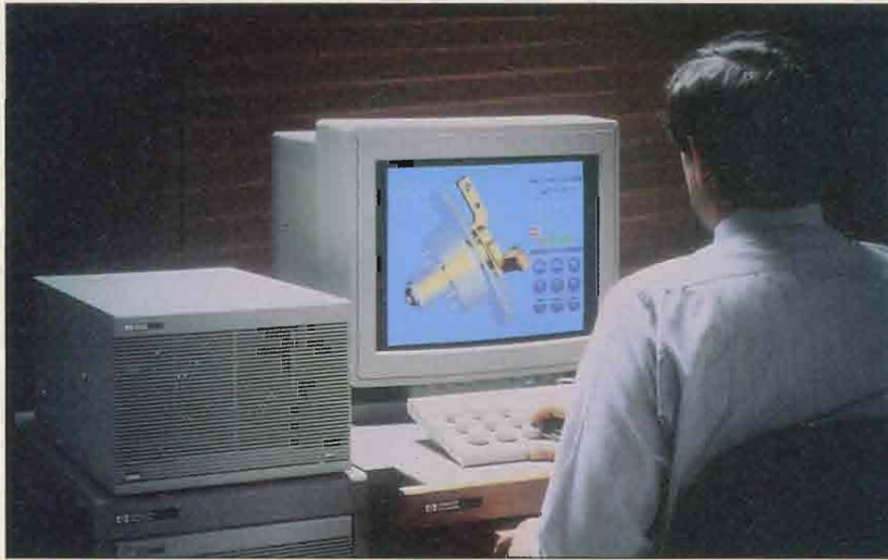
Solid objects can be rendered at interactive speeds with the HP 9000 Model 825SRX, HP's new superworkstation.
