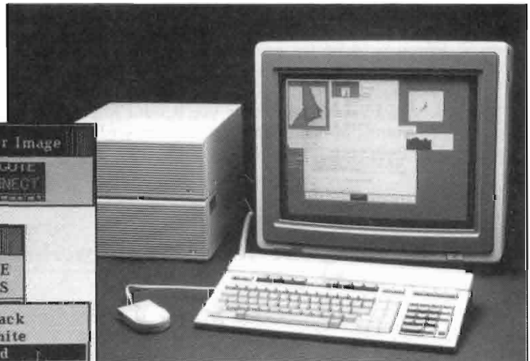
The X Windows System is a screen display and user-interface technique that allows the user to work with multiple applications simultaneously and move data among them.
