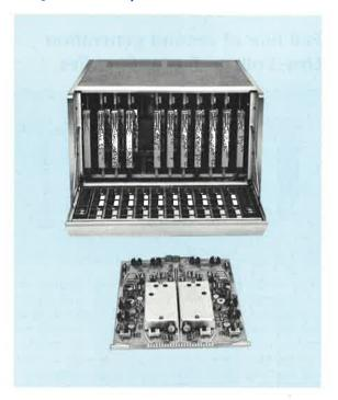
High-speed data acquisition systems can now be equipped with wideband, differential-output, amplifiers at a cost of less than \$400 per channel. This capability is obtained with the new HP **2471A** System Data Amplifier and the price includes 20-channel combining case, power supply, and provision for switching gain and bandwidth.
