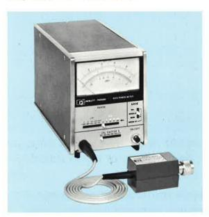
Confidence in system measurement accuracy is provided by the new 437A Thermocouple Power Meter with its exclusive internal calibrator. The front panel calibrator switch automatically compensates for changes in thermocouple sensitivity (from temperature variations, aging or overload) by matching instrument gain to mount sensitivity. Zero setting is also automatic.
