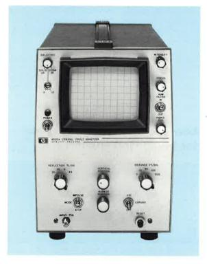
Location and measurement of faults on 75-ohm coaxial systems operating to 300 MHz is easy with the new **4920A** portable Coaxial Fault Analyzer. Using time domain reflectometry, the Model 4920A reads directly in feet with a maximum range of 5000 feet. A times 10 magnification provides excellent distance resolution and measurement accuracy on closely spaced faults.
