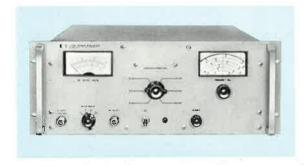
High power and low noise characterize the new HP 230B Tuned RF Amplifier. Like its predecessor, this one covers 10 MHz to 500 MHz in six frequency bands with up to 30 dB of gain and a maximum power output of 4.5 watts, ideal for increasing signal generator output. In addition, lower noise figures, typically 6 to 9 dB, make it suitable for low signal level (preamplifier) applications.
