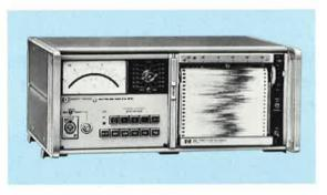
New laws limit employee exposure to excessive noise. To establish compliance you may need acoustic noise levels measured accurately, automatically, continuously and unattended. Use the HP Model 80511P Level Recorder, a combination of an 8052P Precision Sound Level Meter and a 680 Strip Chart Recorder (modified). Detection modes (SLOW, FAST, MAX and PEAK) and weighting networks (A, B and C) are selectable. The built-in log converter provides a linear scale for meter and recorder.
