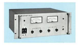
Long established as preferred system supplies for component aging, production testing, and special applications, the LVR Series power supplies now include overvoltage crowbars in all 12 models for protection of delicate loads. Other advantages include low ripple (peak-to-peak as well as rms) and well-regulated constant-voltage/constant-current dc output.
