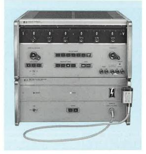
You can get up to 1100 volts from your HP 745A AC Calibrator by adding the **746A** Amplifier. A tenfold increase in output voltage is obtained over the frequency range of 10 Hz to 110 kHz. The 6-place voltage dials on the AC Calibrator still control the output (within  $\pm 0.04\%$  of setting from 50 Hz to 20 kHz) and the benefits of the AC Calibrator—stability, usability, speed, direct per cent error readout, ease of calibration, programmability, and purity of signals—are retained.
