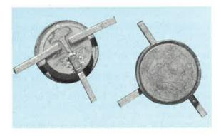
For critical oscillator and amplifier applications to 6 GHz, HP offers hermetically sealed stripline NPN transistors in two configurations. The commonemitter version (35806E) as a linear amplifier typically provides 20 mW output with 5 dB NF at 2 GHz. In a common-base version (35806B), this high performance transistor is ideal as an oscillator; 20 mW output at 4 GHz is typical.
