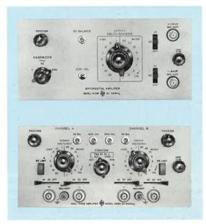
limit switches (5, 50, and 500 kHz in the 1400B and 50 and 500 kHz in the 1408A) improve resolution of low-level signals by eliminating the noise in the unused portion of the bandwidth. With the high degree of stability of these amplifiers, ac-coupling as a means of eliminating drift is not necessary. Prices: 141B, \$1500; 1400B, \$275; 1408A, \$575.
