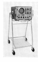
♠ AC-II5B Oscilloscope Testmobile. For ♠ oscilloscopes. 4" rubber tired wheels, heavy chrome tube construction, tilts 'scope to 30° in 7½° increments, folds for storage, shipping.
