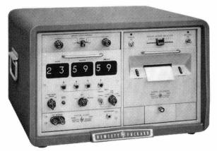
Continuous digital record from p and Dymec counters, voltmeters, other equipment
