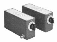
Here are two 50 ohm attenuators providing, together, 0 to 132 db attenuation in 1 db steps from dc to 500 MC! © 355A provides 0 to 12 db attenuation in 1 db steps; © 355B provides 0 to 120 db attenuation in 10 db steps. One simple control for each attenuator; overall full range accuracy is  $\pm$  0.25 db for  $\oplus$  355A. For  $\oplus$  355B, accuracy is  $\pm$  1 db to 250 MC;  $\pm$  2 db to 500 MC. \$\overline{p}\$ 355A or 355B, \$125.00.
