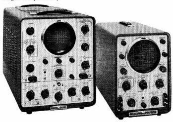
Both instruments have universal automatic triggering where one preset adjustment provides optimum triggering for all conditions. Other features include unitized circuits, etched, mounted on "see-through" plastic; highest quality components, ultra conservative design; concentric color-coded controls, direct sweep-time selection.
