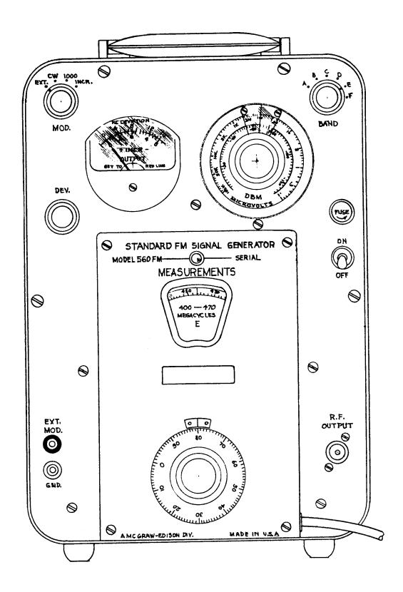
Figure 1. Front View of Model 560-FM Standard Signal Generator
