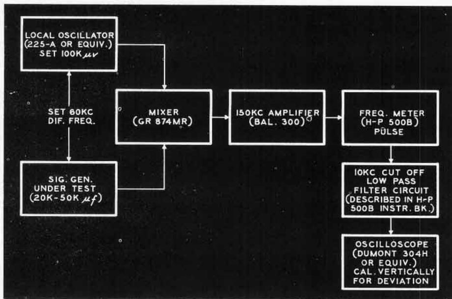
Figure 3. Test set up for measuring incidental FM on the 225-A.
