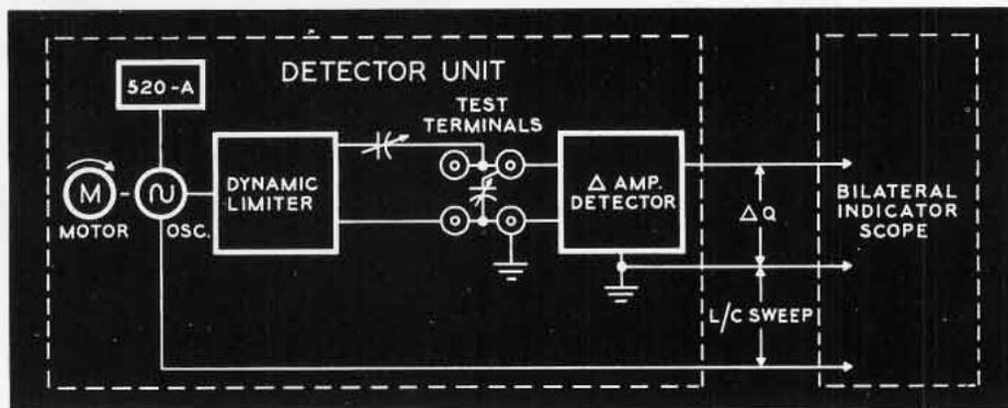
Figure 2. Block Diagram — Q Comparator.
