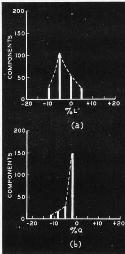
Figure 3. Typical tolerance distribution curves for analyzing pilot and production component runs.
