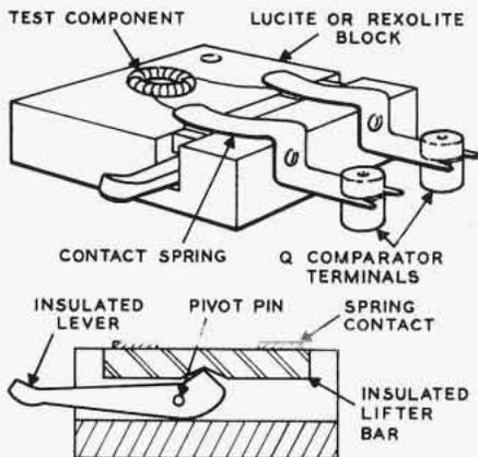
Figure 5. A manually-operated fixture designed to speed up component testing on the Q Comparator.
