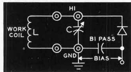
Figure 4. Circuit connections for checking capacitor diodes on the Q Comparator.
